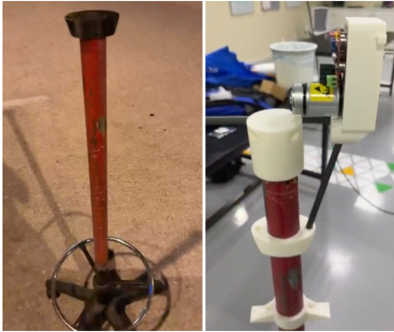
Figure 12: Robot Base (left) and 3D-mounted parts with steel pipes (right).
